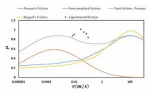
Figure 3: Comparison of klüppel & persson friction models
