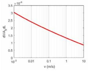
Figure 10: Wear rate vs sliding velocity
