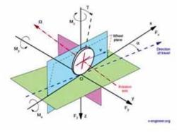
Figure: Tyre axis system and terminology defined by SAE standards (right-hand road wheel)
