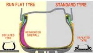
Fig.3: Self Supported Run-flat Tyres have a Reinforced Sidewall
