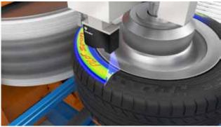
Gocator 2530 high speed 3D blue laser profiler scanning a tyre sidewall
