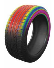
Laser profile sensors provide an ideal solution to both in-process and final rubber and tyre measurement and quality control applications. Built-in measurement tools for strip positions, including multiple groove location and depth measurement monitoring with automated alignment enable engineers to configure setup parameters—without requiring any measurement software development.
