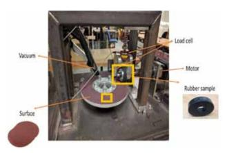
Figure 11: Dynamic friction tester
