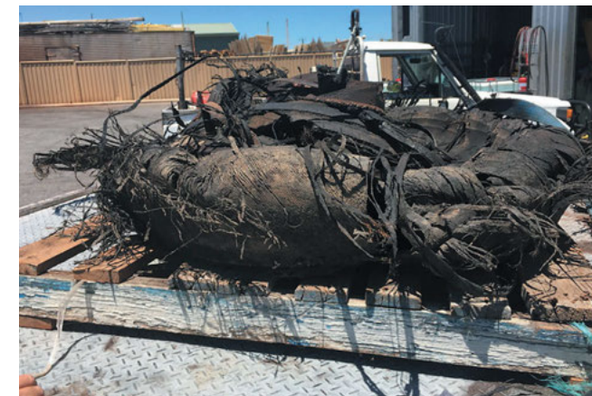
Catastrophic steer tyre failure.
