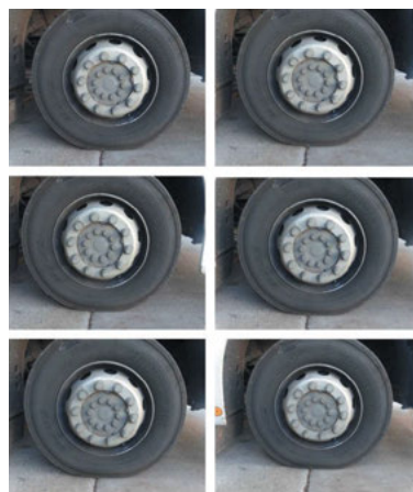
A 295/80R22.5 steer tyre, reduced by 10psi from 120psi to 60psi. When is it flat?
